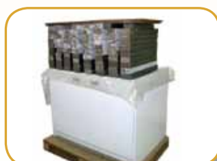
Actual photo during Cabinet Load Testing
